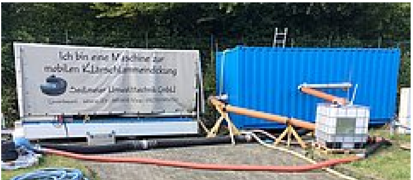
Fig. 1: Validation operation - a pump sump was retrofitted into an existing buffer tank with concrete shaft segments. The demonstration plant HUBER Drum Screen LIQUID is fed with the effluent from the mechanical pre-treatment system. The effluent (screened wastewater) of the LIQUID machine flows by gravity back into the buffer tank
