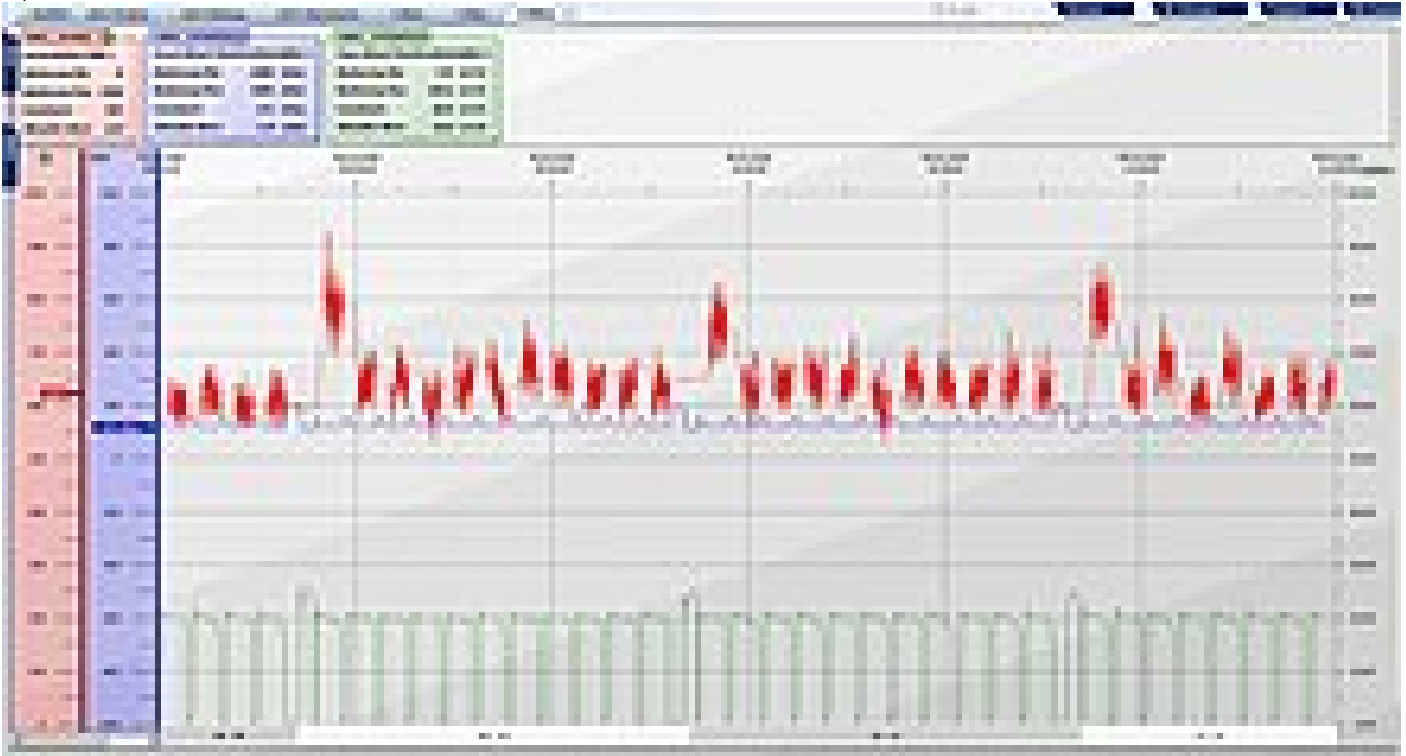
Fig. 7: Part of the process control system, visualisation of the membrane filtration plant ; red: permeability curve
