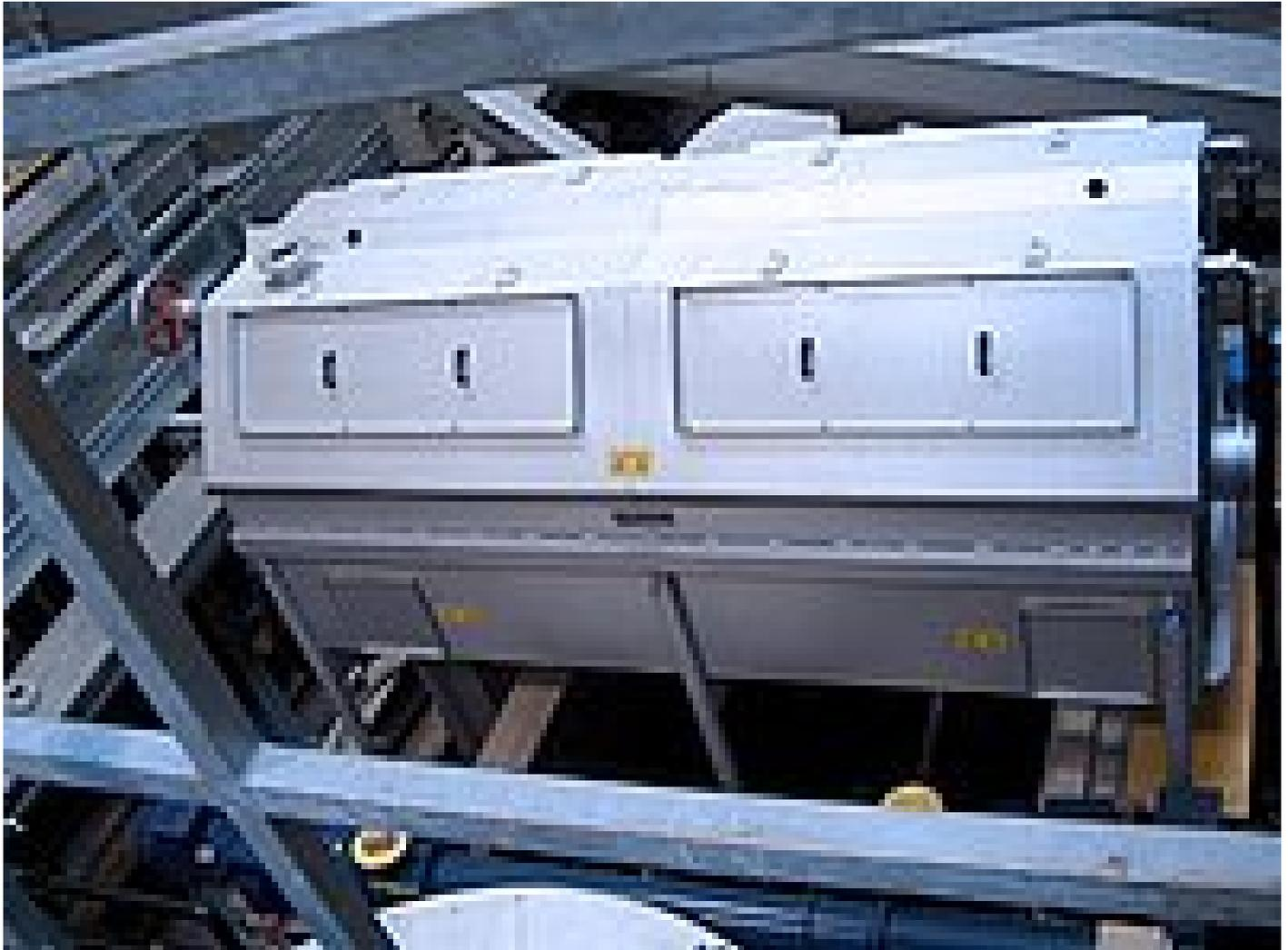
Ultra fine Rotary Drum Screen with two-dimensional effect for very fine particulate material
