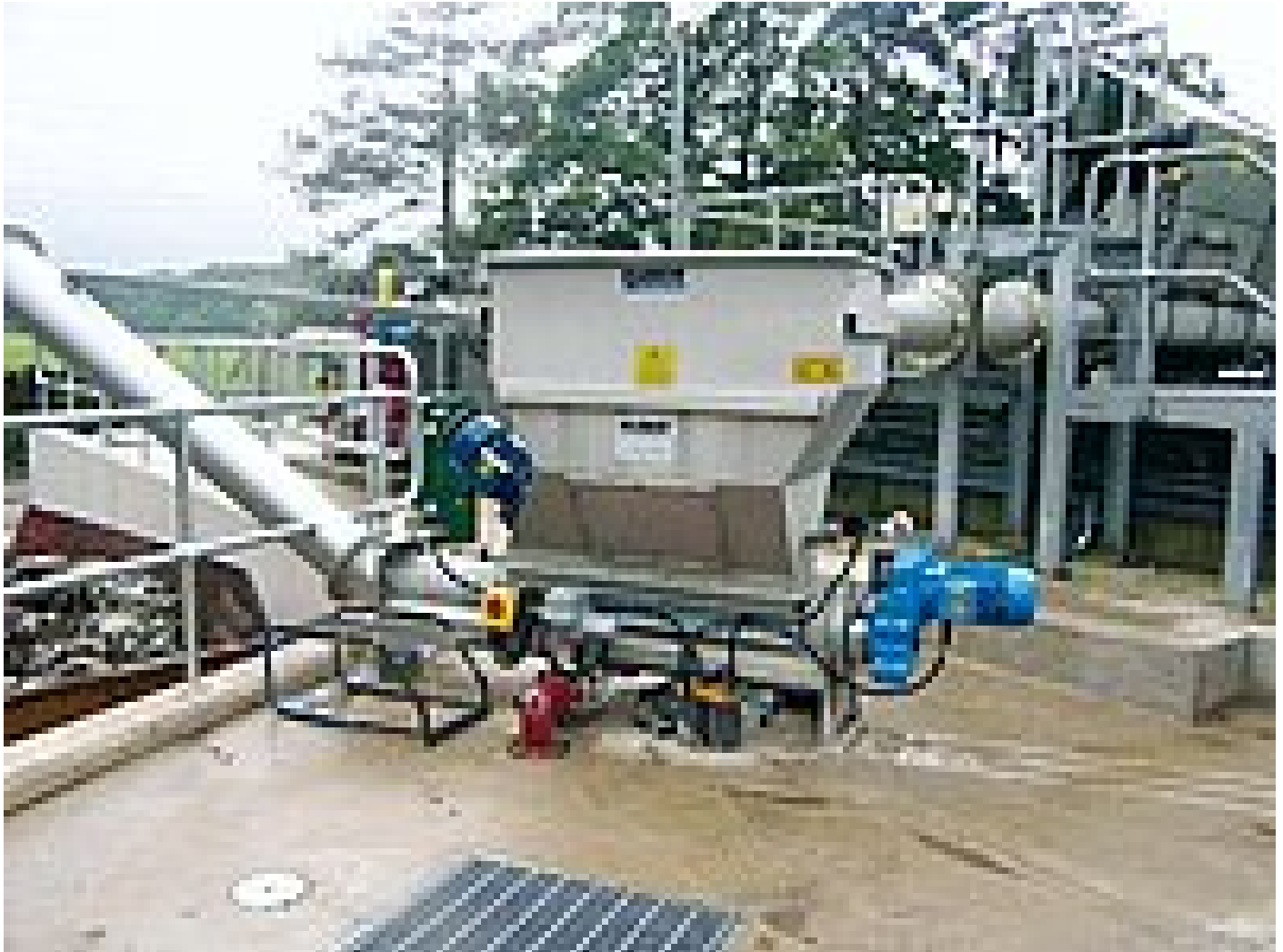
The HUBER super-laundry wash-press WAP/SL is fed through a launder channel
